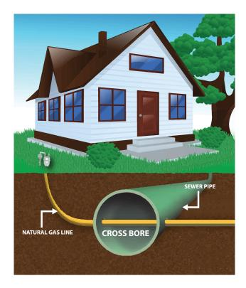
If a cross bore exists, and you or your contractor use a mechanical rotary device (auger) or hydro-clearing device to root out the blockage, a serious safety risk could result. In the event of a blockage, ask your contractor to use a <u>camera</u> to determine the condition causing the blockage.
