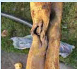
Pipe damaged by lightning strike
