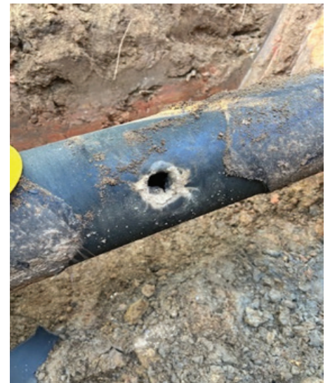
Damage to a 6” steel natural gas pipeline from a bore operation installing broadband fiber cable shut down Highway 5 in York for two days.
